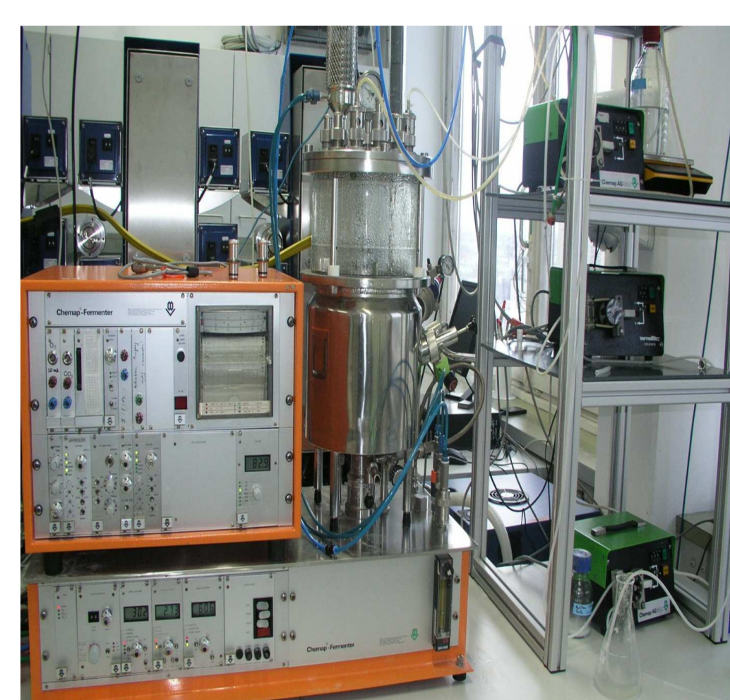
Fermenter for glucose fermentation by S. cerevisiae for the production of bioethanol and CO 2 .
