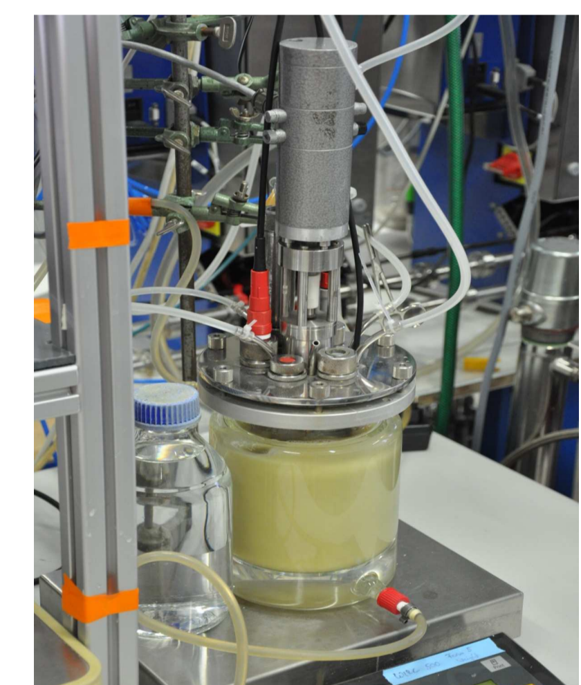
Fermenter for biomethane production using pure culture of a thermophilic methanogenic strain
